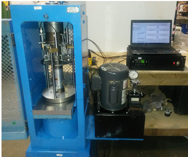
Figure 1: Forney loading frame setup for UCS testing.
